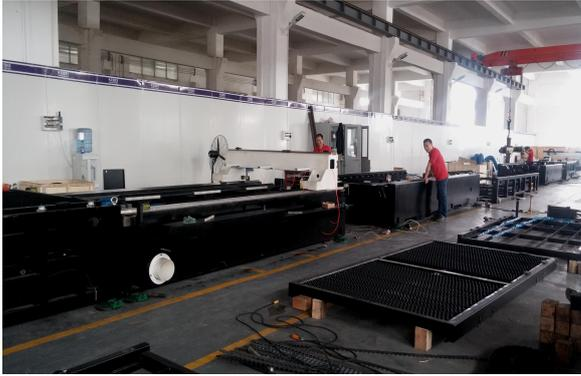
1 Our gantry-type flying optical path structure working table has been annealed to relieve internal stress strictly, thus significantly improves the rigidity and stability of the CNC laser cutter.
